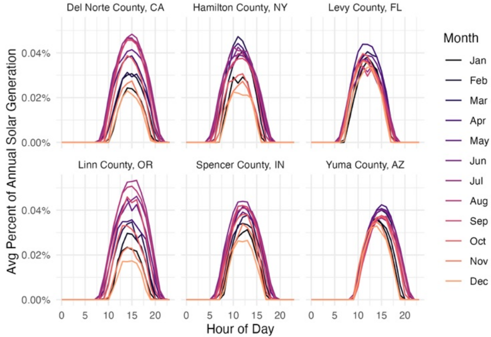
Figure A2: Hourly electricity generation for a standard solar panel for six example counties.
